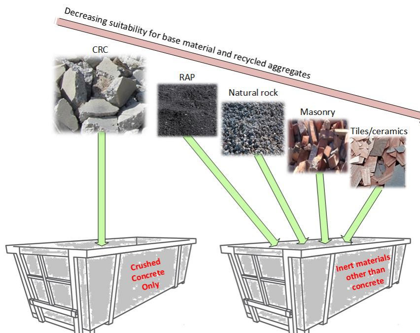
Figure 9 - Source separation of comingled C&D for base material and recycled aggregates
